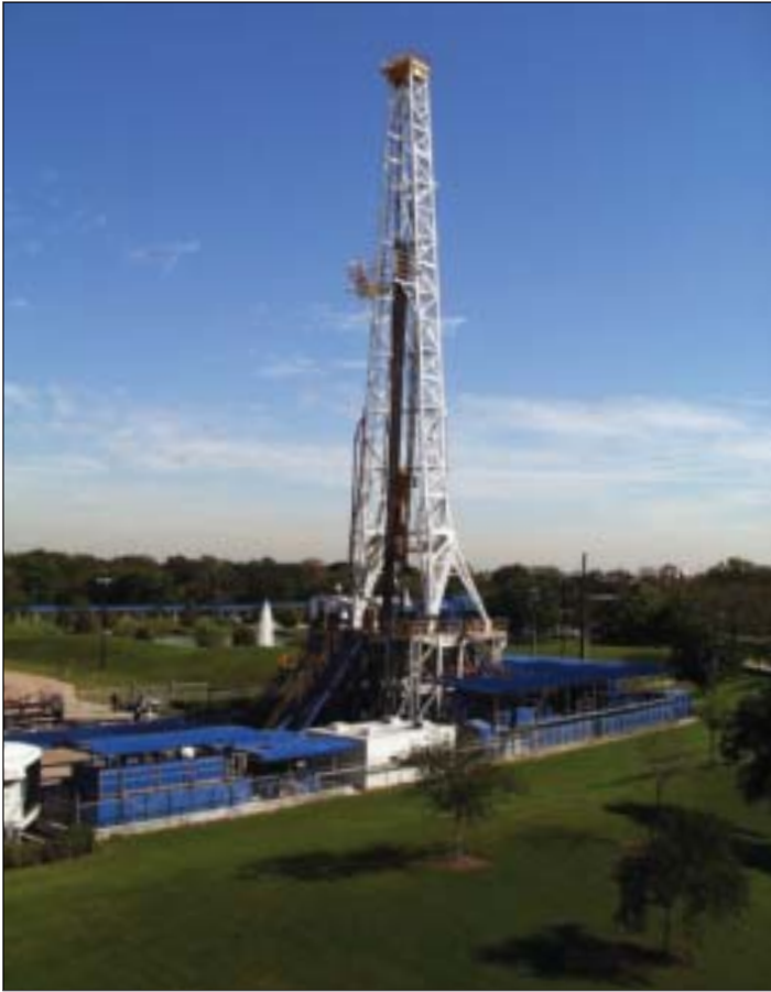
^ Genesis Drilling Test Facility. Genesis is a 142-ft [43.3-m] cantilever-type, skiddable land-drilling rig with 1,250,000-lbf [5,560-kN] derrick capacity. In service at the Sugar Land Technology Center since 1988, Genesis is used to reproduce downhole field conditions for various types of tests. Mud flow, pressure, shock, vibration and rotation of downhole tools can be performed under controlled conditions, either by drilling through cement or by using a shock-inducing device, also known as cam sub.
